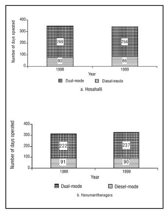
Figure 1. Number of days biomass gasifier system operated on diesel and dual-fuel mode in Hosahalli and Hanumanthanagara during 1998 and 1999.
